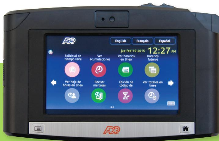
In addition to Web, interactive voice response, and mobile data collection options, ADP offers intelligent devices that capture employee time using badge, smart card, proximity, barcode, PIN or biometric technology. All available languages are offered on a single timeclock to accommodate a diverse workforce.
